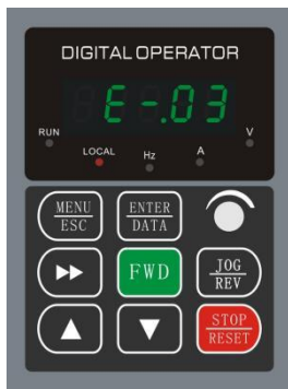
Fig. 4-5 Fault alarm display state
