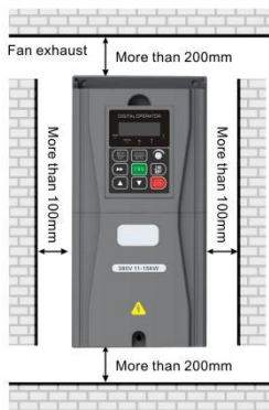
Figure 3-1 Mounting space and distance
