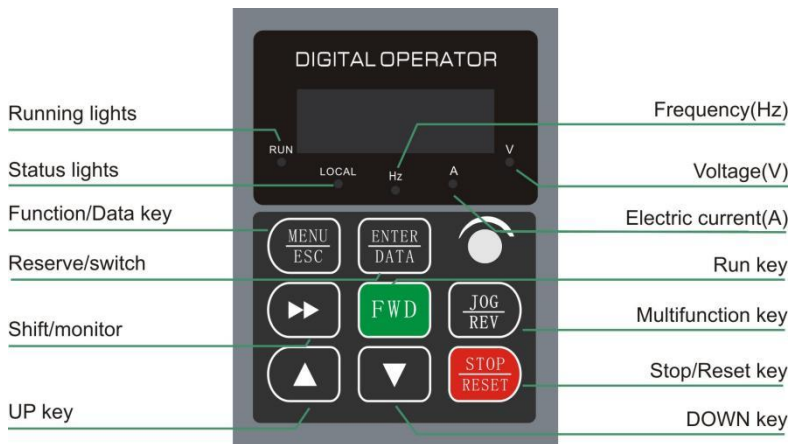
Fig. 4-3 Control panel diagram
